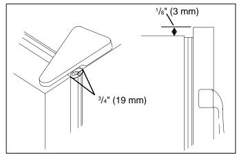
Remove plugs from side of refrigerator and freezer doors using a putty knife with the blade covered in masking tape.
